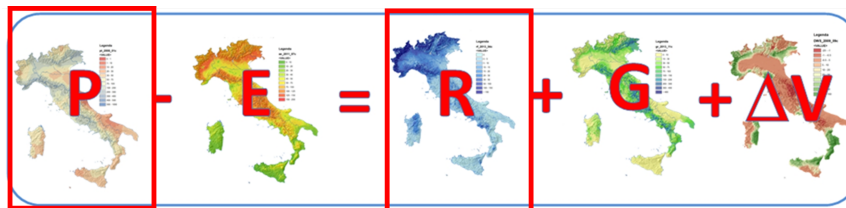
Figure 3.2: Figure shows selected components for the study from BIGBANG dataset such as total precipitation (P) and surface runoff (R) to support runoff coefficient and aggregated runoff calculations for rainwater harvesting potential assessment along with other variables, evapotranspiration (E), aquifer recharge (G) and soil/snow water storage ( \Delta V )
