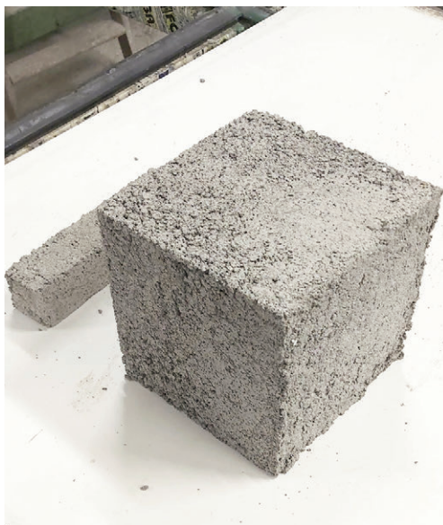
Fig. 4 | Cubic concrete test specimen (15 cm side) with replacement of fine aggregates by the recycled glass (credit: the Authors, 2023).
