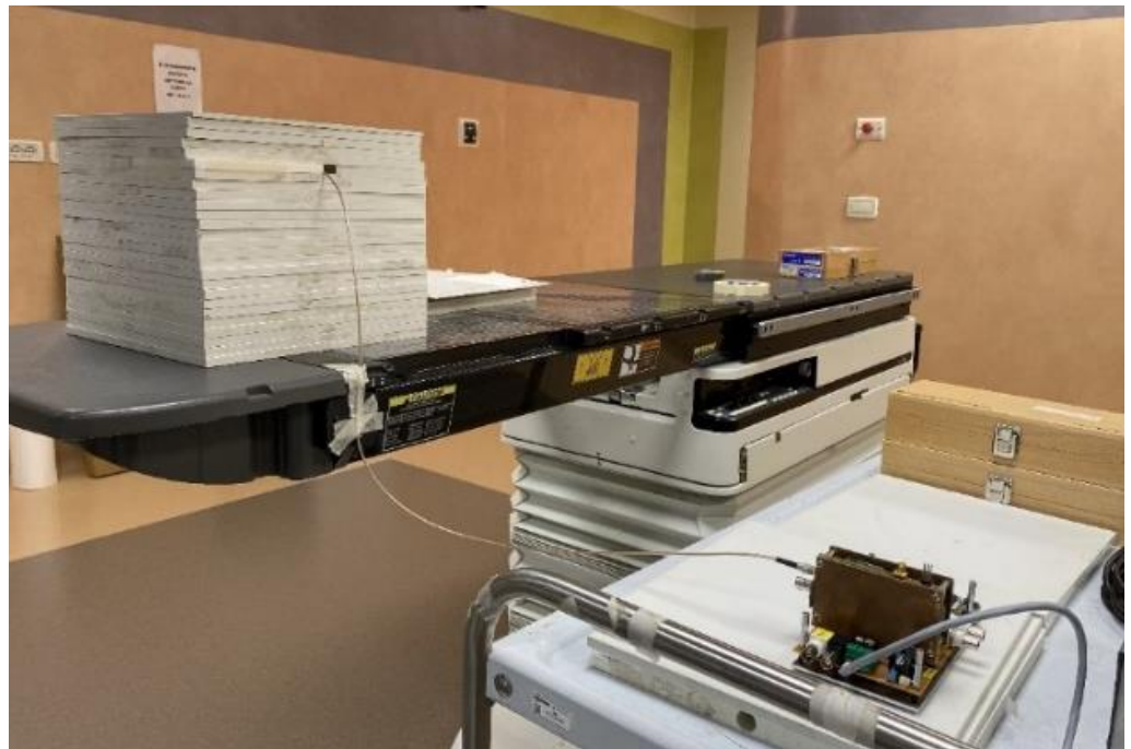
Figure 4. Picture of the characterization setup under high-energy pulsed X-rays. The dosimeter, placed inside a solid Plexiglass ® phantom (on the left), is positioned at the isocenter of LINAC, under a 10 \times 10 \text{ cm}^2 field.
