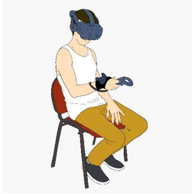
Figure 2. Illustration of an individual equipped with all the sensors employed in the study, posed to initiate the task within the experimental setup. The person is wearing the headset, is holding the controller with their right hand, and has the tracker attached to their right wrist.
