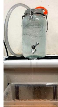
Fig. 5. Experimental hydraulic setup used for measuring the collected water mass over time.
