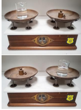
Fig. 4. Balance used to assess the accuracy of mass measurements achievable in Galileo's time.
