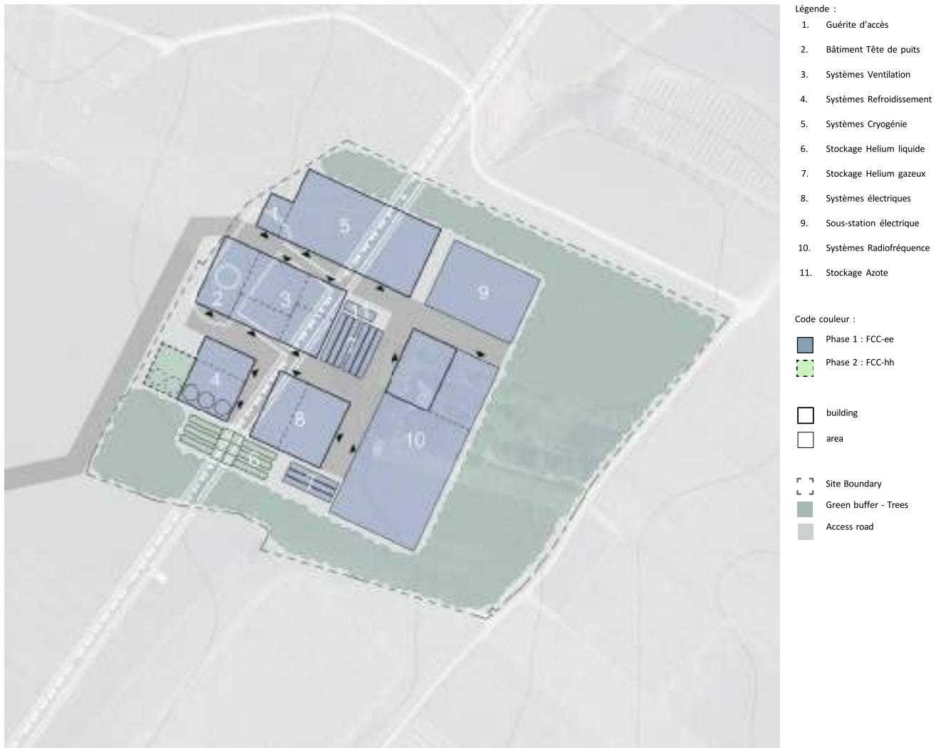
Fig. 2.71 Space requirements for a site integration of technical site PL in Challex, France
