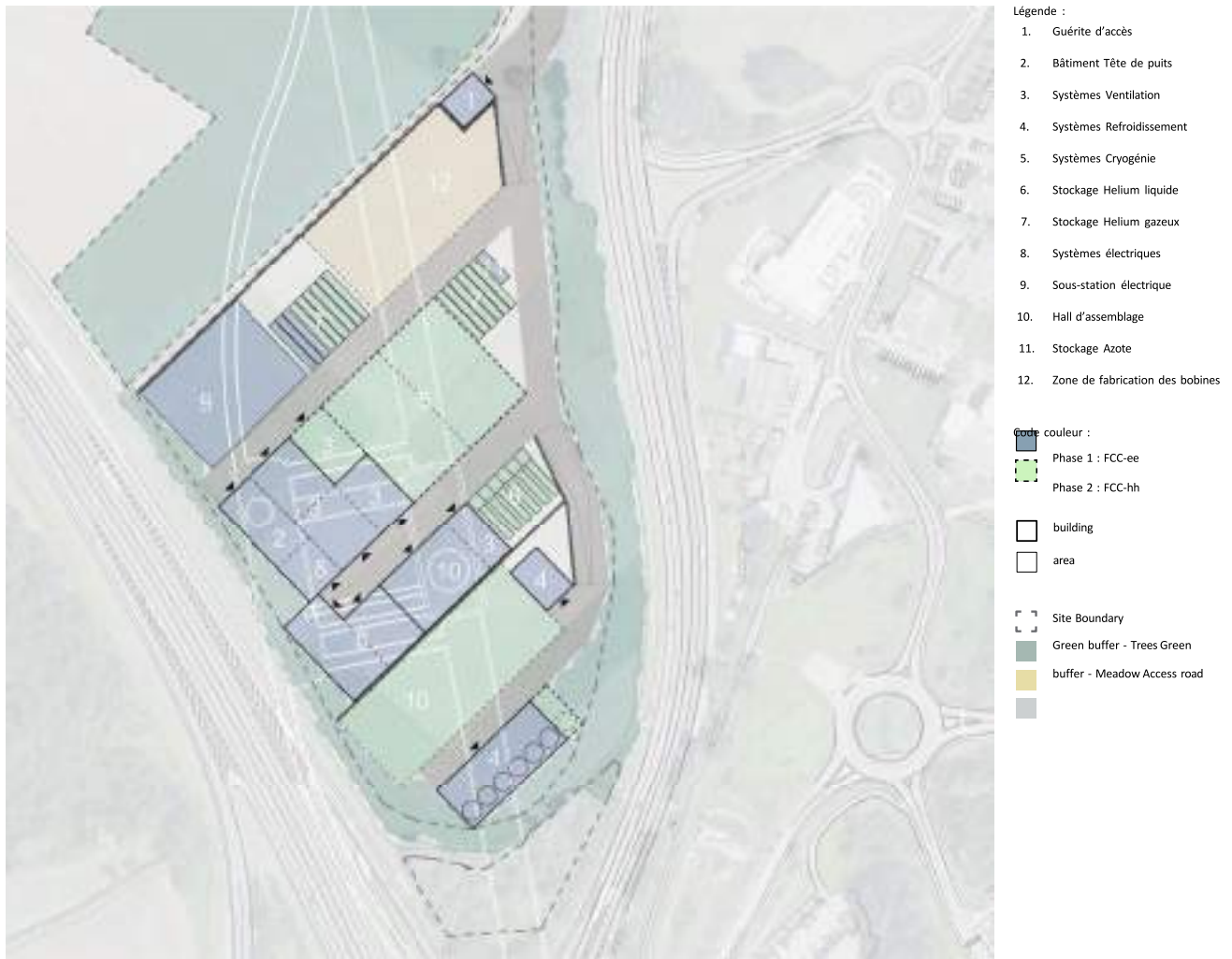
Fig. 2.66 Space requirements for a site and landscape integration of experiment site PD in Nangy, France
