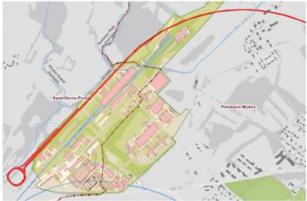
Fig. 2.48 Sketch of the current working hypothesis for a linear-accelerator based injector that has a length of about 1.2 km. A definitive placement remains to be developed in the frame of a design phase, considering environmental, existing experimental facility, territorial development and engineering constraints
