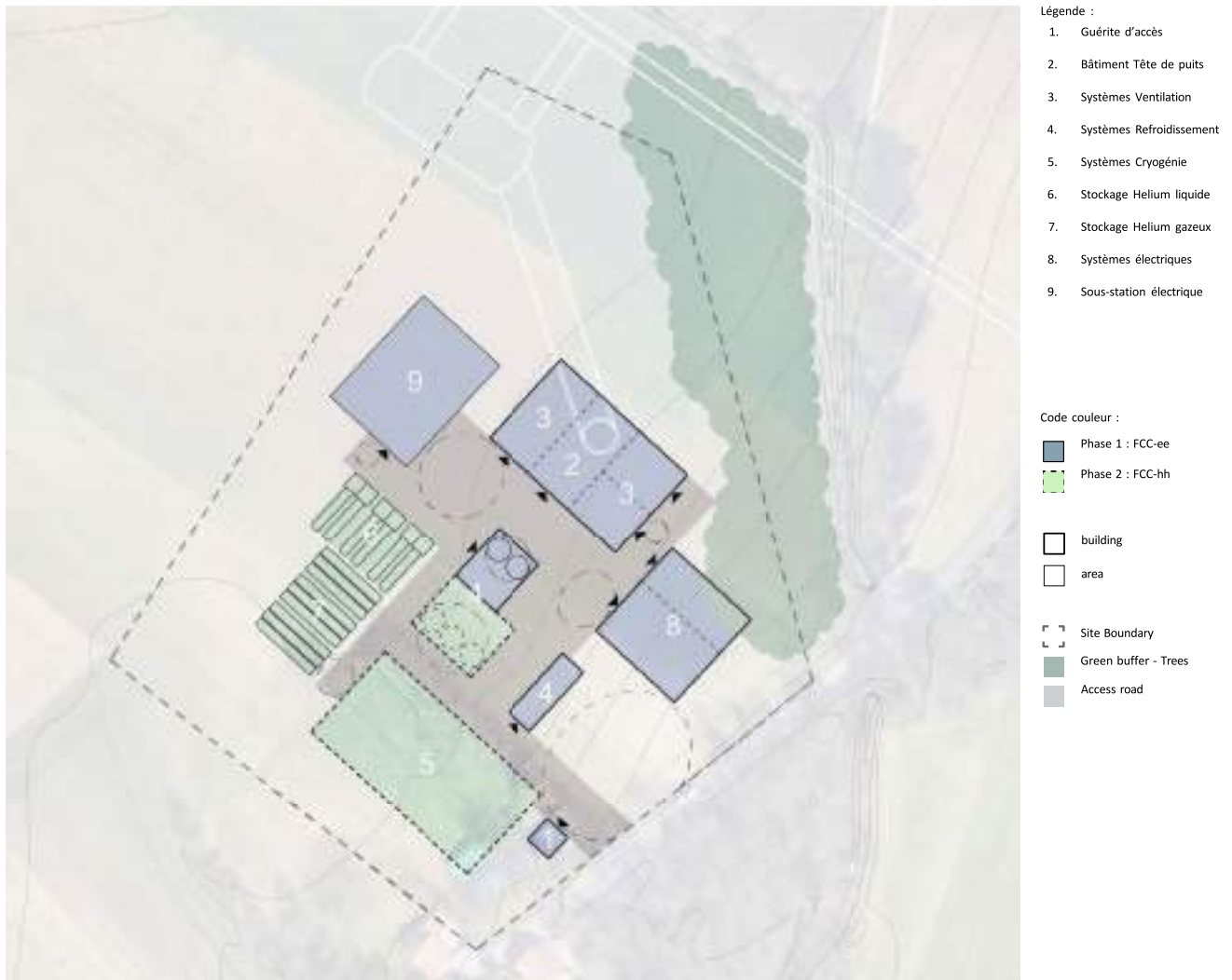
Fig. 2.65 Space requirements for a site and landscape integration of experiment site PB in Presinge, Switzerland
