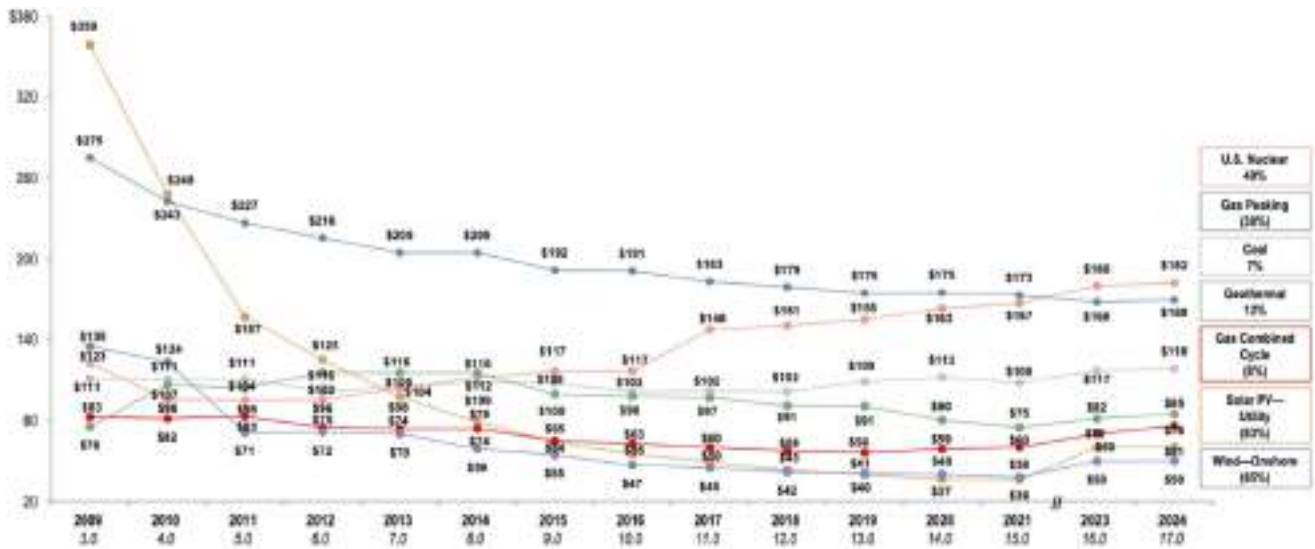
Fig. 3.4 Evolution of the levelized cost of electricity (LCOE, Source: Lazard's Levelized Cost of Energy Version 17.0)
