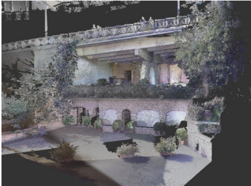
Figure 3.1: Raw point cloud of the Zagarolo bridge with in the urban context
