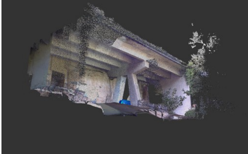
Figure 3.2: Intermediate cleaning step: focus on the bridge area with residual context
