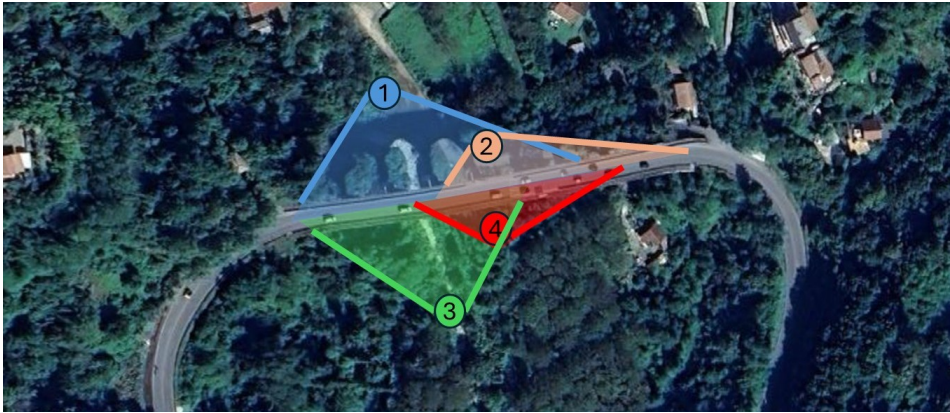
Figure 5.16: Positions of stations of Terrestrial Laser Scanner
