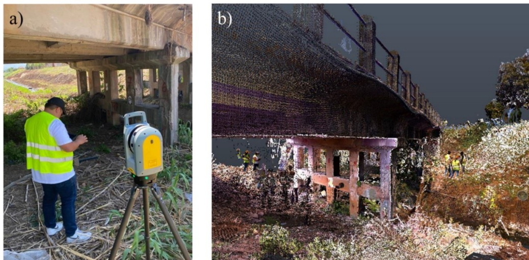
Figure 2.5: a) Setup of laser scanner, b) Acquired point cloud
