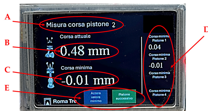
Figure 7. The measurement screen contains information relating to the piston being measured: (A), the current piston stroke (B), the minimum stroke recorded so far (C), and the minimum stroke values recorded for previously measured pistons (D). Touch buttons for performing specific operations during the measurement (E).
