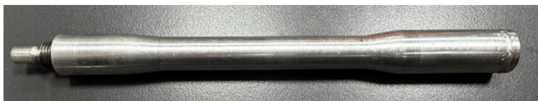
Figure 3. Central body, threaded end, and connection element.
