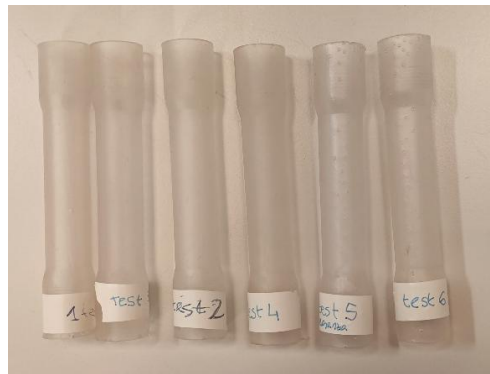
Figure 3.13. Cylindrical specimen 3D printed using SLA, obtained from the average cross-sectional dimensions of the trachea.
