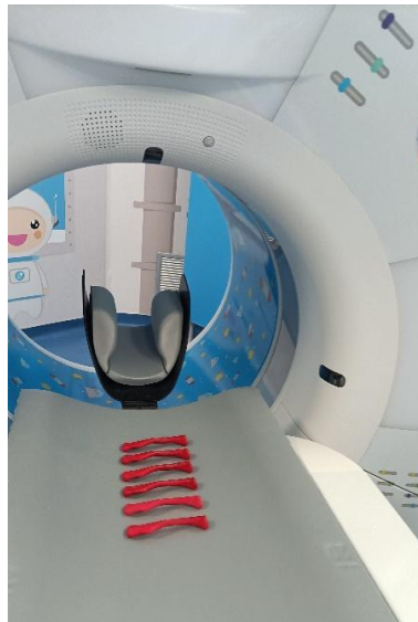
Figure 4.7. Setup for CT-D acquisition of the six 3D-printed clavicle replicas with Siemens Somatom Force.
