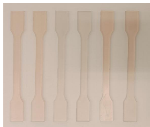
Figure 3.14. ISO 527-1A dog-bone specimen 3D printed using SLA, included as a standardized reference geometry for comparative mechanical assessment.
