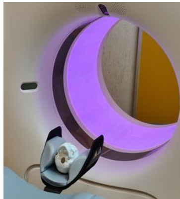
Figure 4.3. Cranial model 3D printing centered within the gantry using a cruciform laser system.
