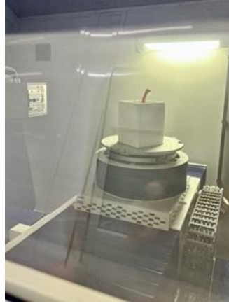
Figure 4.9. CT-I scan of a single model with ZEISS METROTOM 1500.
