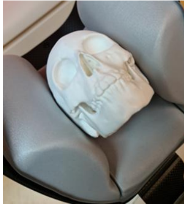
Figure 4.2. Cranial model 3D printing placed in the dedicated stand for CT scan.
