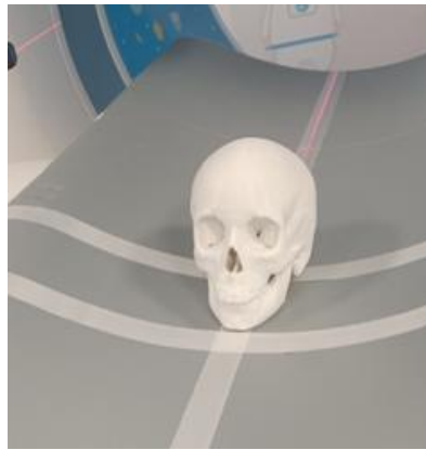
Figure 4.5. Alignment and orientation of the models on the CT patient table
