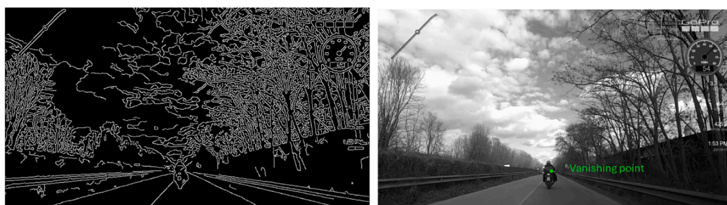
Fig. 3. Canny edge detection (left) and output of vanishing point detection (right).
