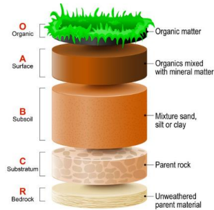
Fig. 1 Geological structure of a soil (Soil is the thin layer of material covering the earth's surface.)
