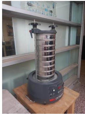
Fig. 15 A sieve used for sifting soil. The sieving time was set to 12 minutes to sift the different grain sizes evenly.
