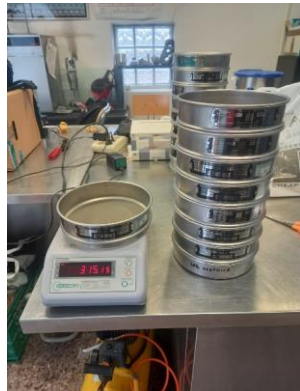
Fig. 16 Gross weight weighing operation sieve with soils inside.
