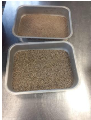
Fig. 14 Fine sand sample at the top and coarse sand sample at the bottom.
