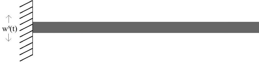
Figure 1: The cantilever beam under support vibration
