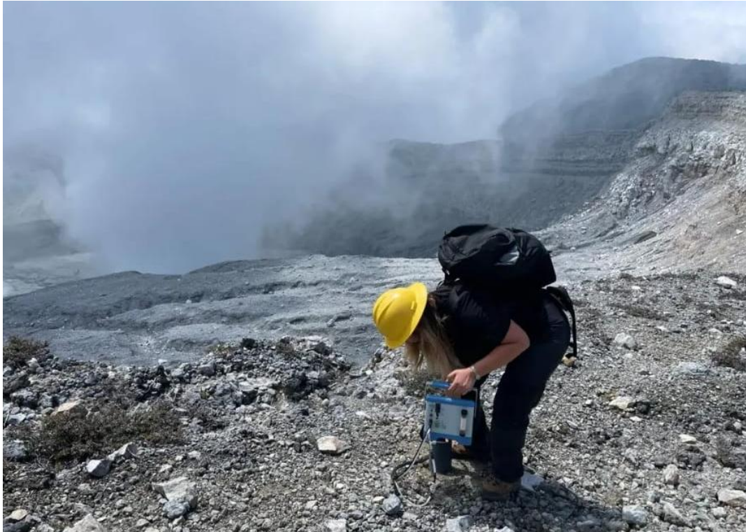
Figure 6.4 - CO 2 measurements along the crater rim at Poàs Volcano (Costa Rica).
