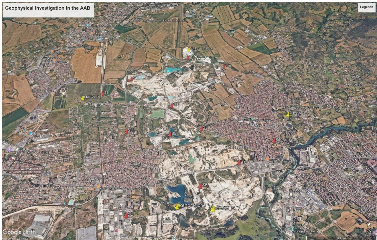
Figure 2.18- MASW location (yellow points) and geophones location (red points) for the geophysical investigation of the Basin.
