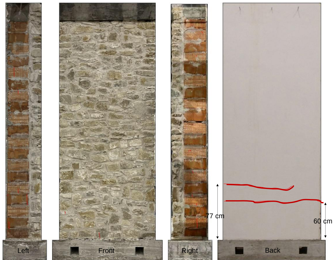
Figure 5. Damage pattern at the end of the seismic sequence with scale factor 2.2.
