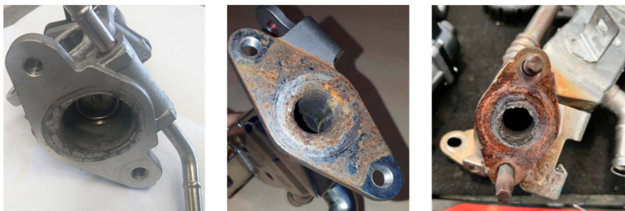
Figure 2. Examples of EGR coolers that are affected by chlorine corrosion; the three cases shown relate to increasingly severe degrees of corrosion.
