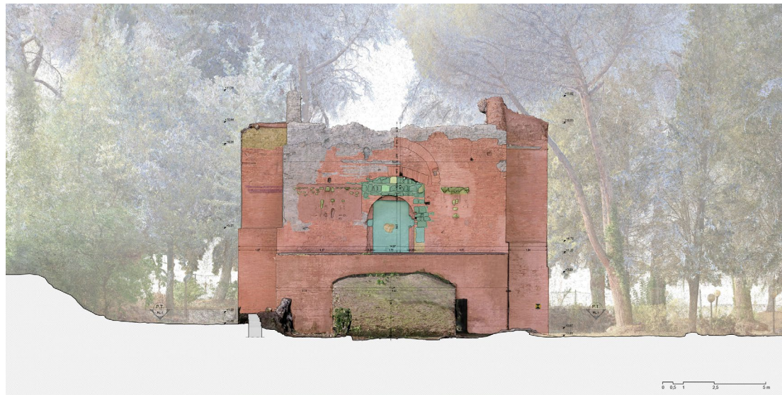
Fig. 13 - Transverse section 44': integration of vector-based CAD drawing with orthophoto (graphic elaboration by the authors).
