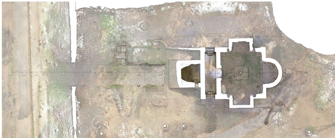
Fig. 10. Floor plan of the Mausoleum of Sant'Urbano: integration of the CAD vector representation with the orthophoto (graphic elaboration by the authors).
