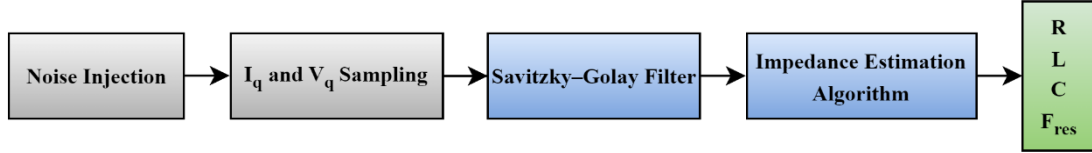
Figure 11 - Impedance estimation method flowchart.
