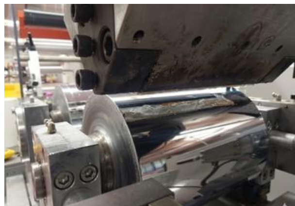
Figure 1.27 Material accumulation at the die during the extrusion of B-PHBH1
