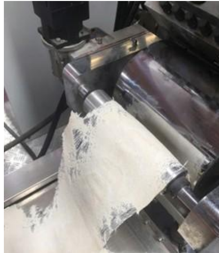
Figure 1.25 Cast extrusion of B-TPS1 sheets with thickness below 120 \mu\text{m}
