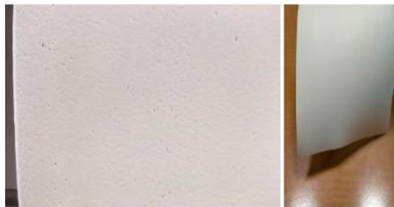
Figure 1.24 B-TPS1 cast extruded sheet. Left: defects related to humidity; right: sheet after the parameters optimization
