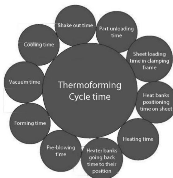
Figure 3.28 Schematic representation of thermoforming cycle time [130]
