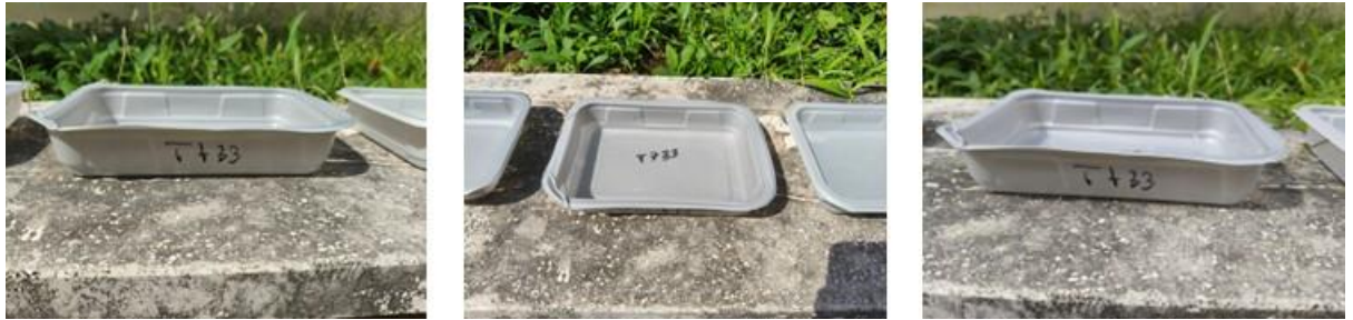
Figure 5.28 Thermal resistance test of T733 trays. From left to right: before, during and after the test.
