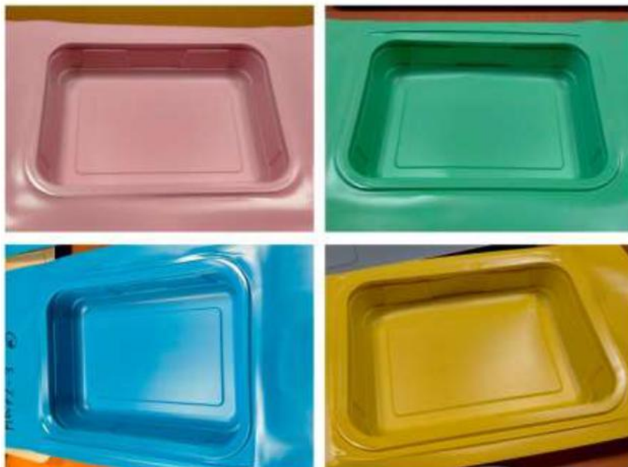
Figure 1.21 Top view of the colored thermoformed trays
