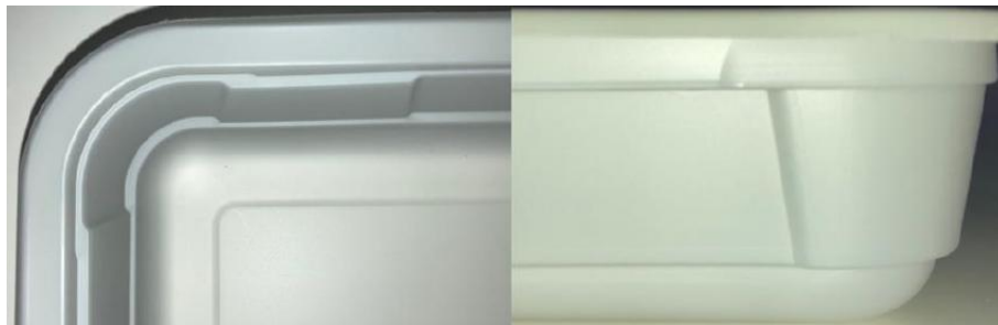
Figure 1.11 Details of the thermoformed trays based on PLA and PBS.
