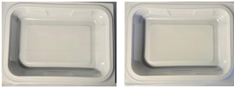
Figure 1.33 Food trays thermoformed from F_T1 sheet (left) and F_T2 sheet (right) [11]
