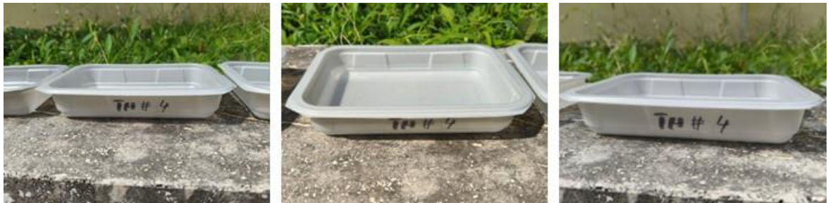
Figure 5.25 Thermal resistance test of PLA-PHBH 82 trays. From left to right: before, during and after the test.
