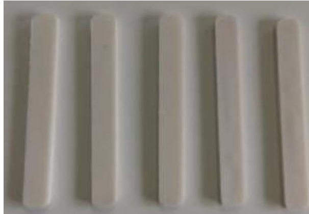
Figure 1.6 Izod samples produced via Injection molding using the SI LA3CL2 formulation
