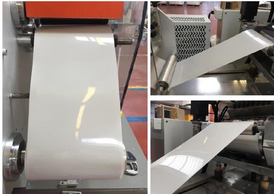
Figure 1.10 Cast extrusion of the formulations based on PLA/PBS
