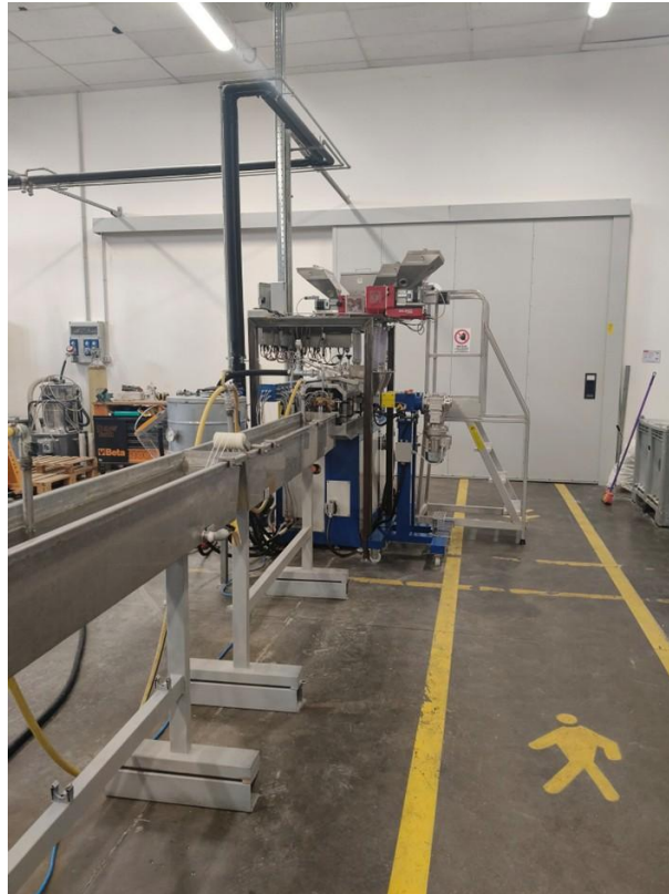
Figure 3.14 COMAC 26 extrusion system
