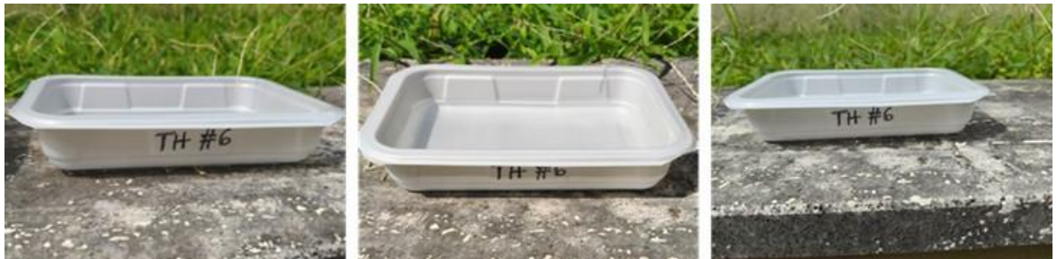
Figure 5.26 Thermal resistance test of PLA-PHBH 55 trays. From left to right: before, during and after the test.
