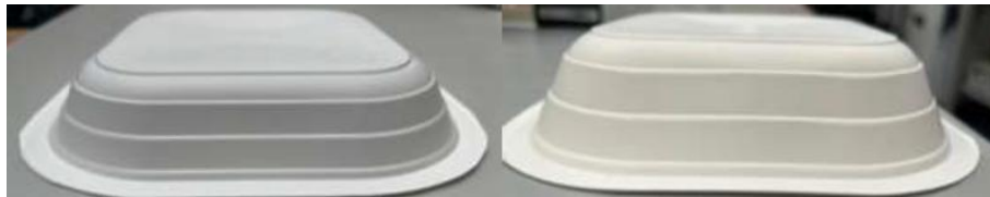
Figure 1.5 Thermoformed trays obtained using the PLA-based formulation
