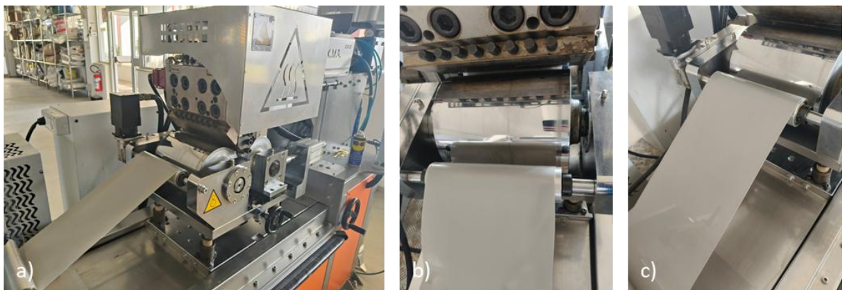
Figure 3.27 Cast extrusion process: a) overview of the extruder, b) sheet of T733 after the calender, and c) sheet of T734 after the calender.
