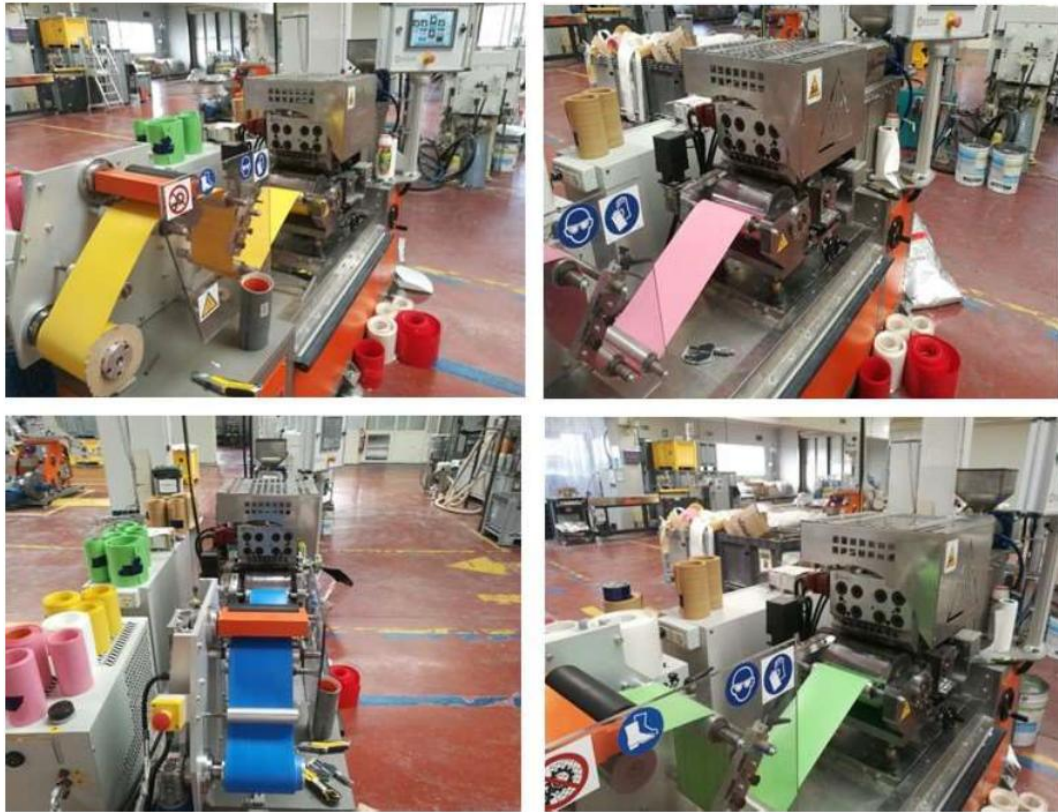
Figure 1.17 Cast extrusion process of the colored sheets
