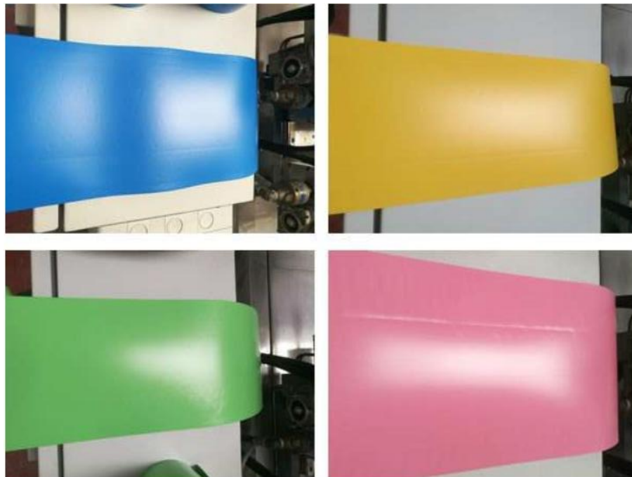
Figure 1.18 Aspect of the colored sheets after the extrusion process
