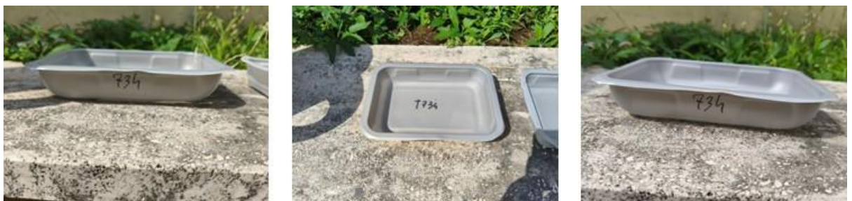
Figure 5.29 Thermal resistance test of T734 trays. From left to right: before, during and after the test.
