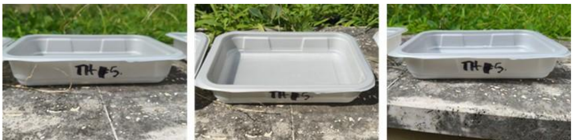
Figure 5.27 Thermal resistance test of PLA-PHBH 28 trays. From left to right: before, during and after the test.
