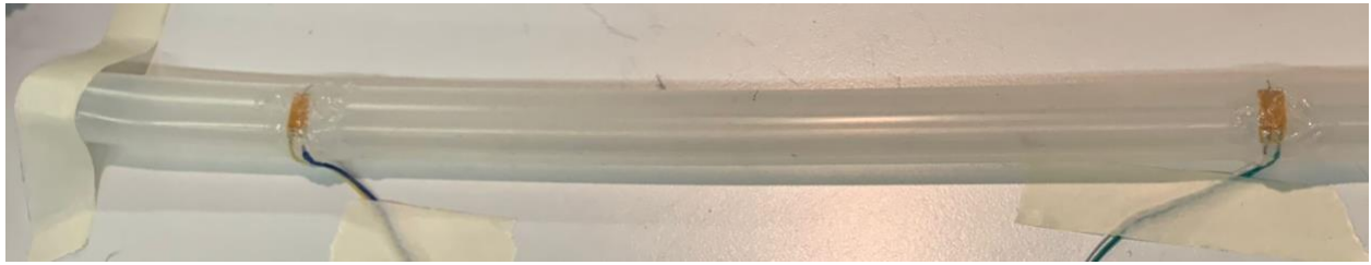
Figure 2.4. Arterial surrogate used within the variable-stiffness simulator during the installation of the sensing instrumentation for detecting the passage of the pressure wave.
