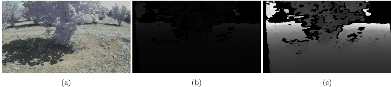
Figure 11: Example of RGB image (a) and respective raw (b) and normalized (c) depth map.
