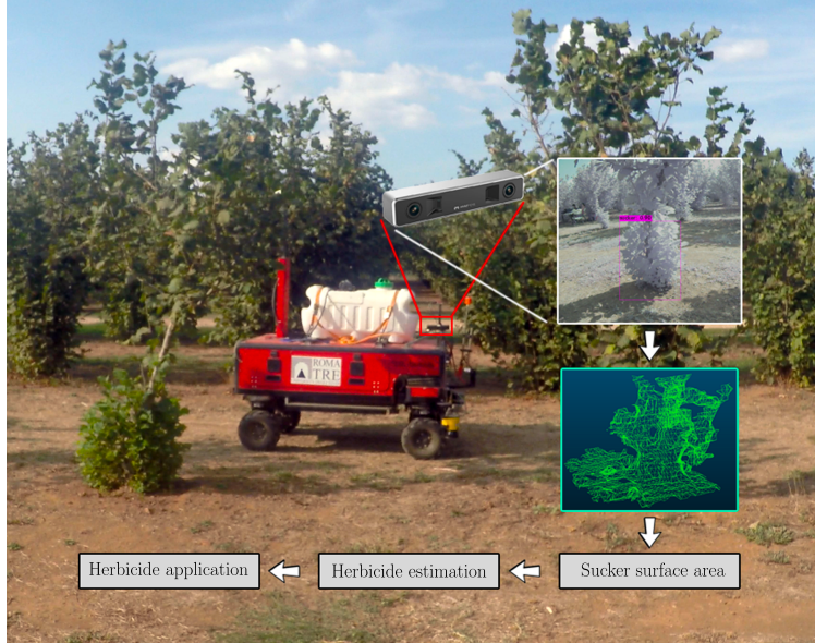
Figure 1: Overview of the proposed autonomous sucker management architecture: each sucker is detected and reconstructed, its surface area is computed and, based on this, the needed amount of herbicide is estimated and applied.
