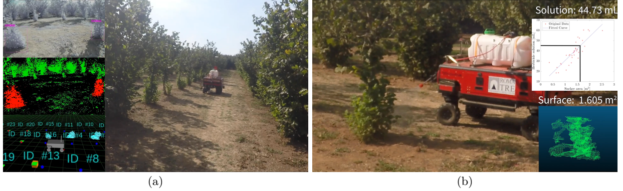
Figure 12: Screenshots of the video showing in (a) the robot inspecting the trees, detecting suckers and reconstructing them, and in (b) the robot spraying a sucker.
