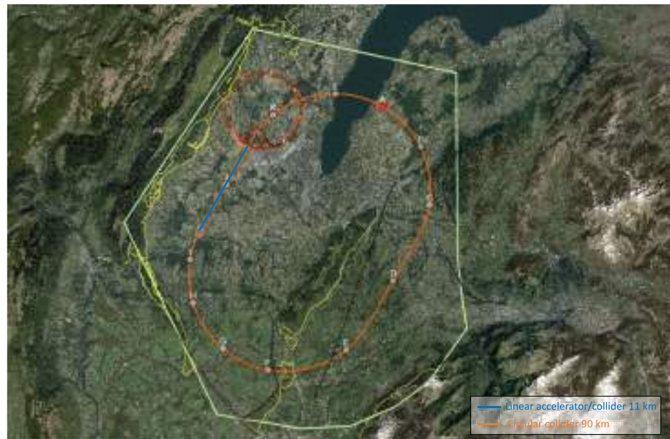
Fig. 2.22 Placement option for a 90 km circular / 11 km linear racetrack scenario
