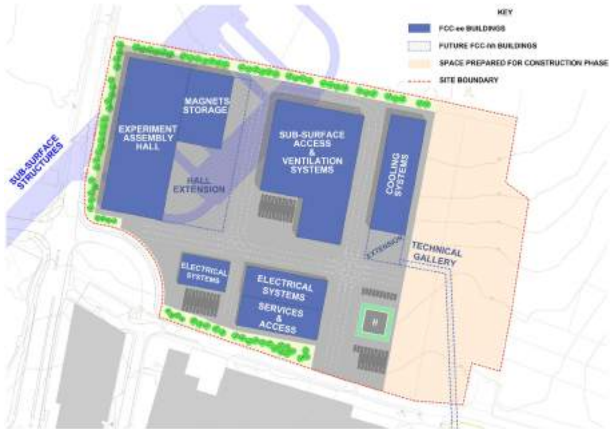
Fig. 1.21 Preliminary simplified surface requirements for PA site
