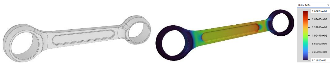
Figure 57. a) Starting CAD model (AS-IS); b) FEM analysis of the CAD model (AS-IS): Load case ID 1, Von Mises Stress distribution.
