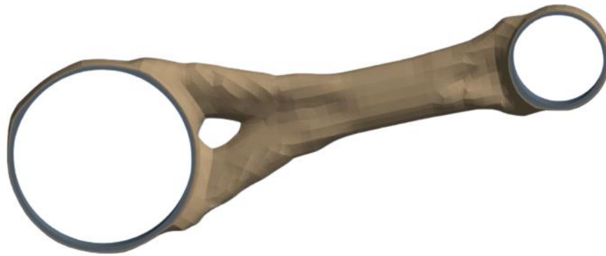
Figure 52. Topology Optimisation Result.
