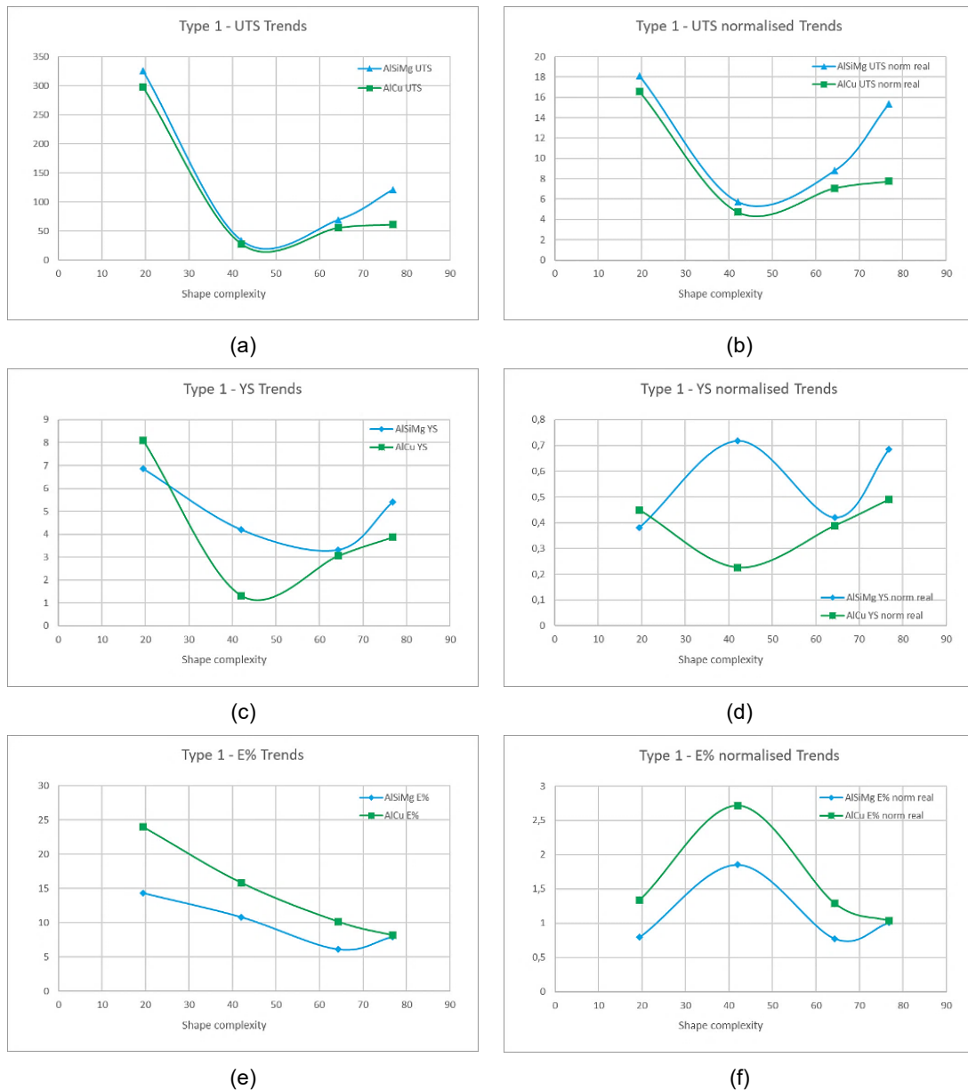
Figure 41 . Type 1 trends and normalised trends: (a) UTS; (b) UTS normalised; (c) YS; (d) YS normalised; (e)E%; (f) E% normalised.
