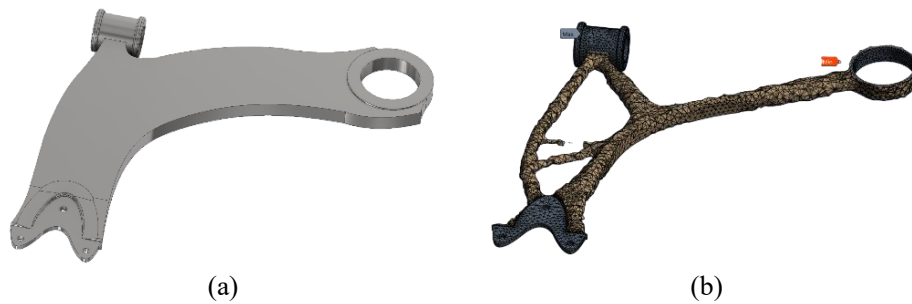
Figure 73. a) Simplified CAD geometry used for the TO analysis, b) Result of TO with 0,4 density value as threshold.
