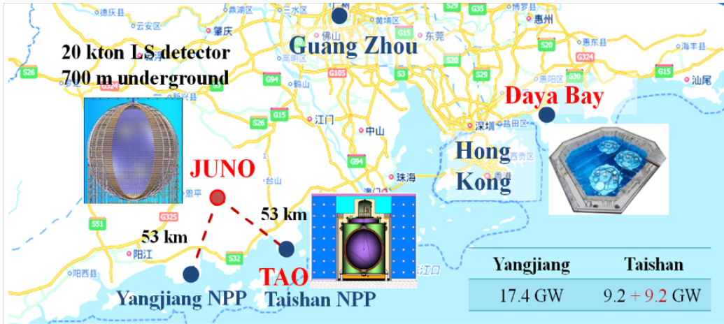
Figure 2.1: Location of the JUNO and TAO experiments in South China. The main 20 kton LS detector, JUNO, is located 700 m underground at a baseline of \sim 52.5 km from six 2.9 GW thermal power (GWth) reactor cores in the Yangjiang NPP and two 4.6 GWth cores in the Taishan NPP. The 2.8 ton JUNO-TAO detector is located about 44 meters away from one of the Taishan reactor cores.
