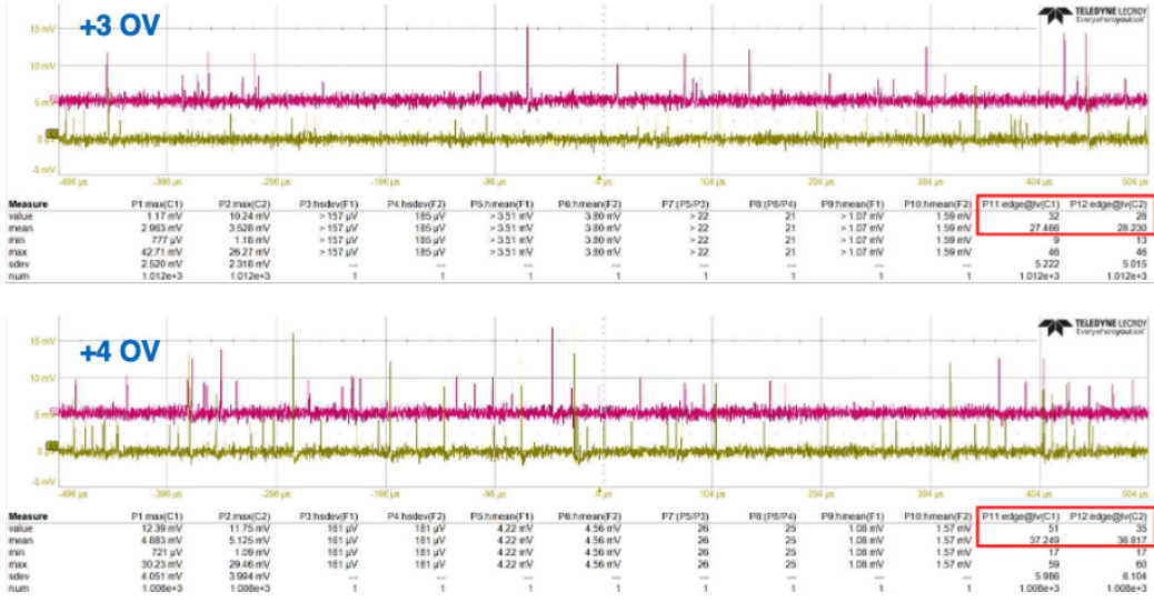
Figure 3.27: Measurement of the dark count rate through the digital oscilloscope, at V_{OV} = 3V and V_{OV} = 4V overvoltages, at -50^\circ\text{C} .
