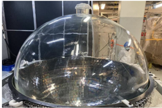
Figure 2.12: Pictures of the installation of the acrylic sphere inside the copper shell.
