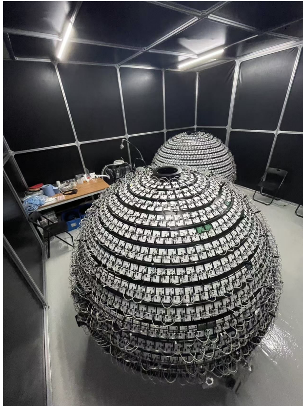
Figure 2.11: Picture of the installation of the 4024 Front-End boards tiles outside the copper shell.
