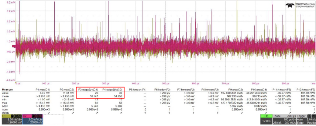
Figure 3.21: Visualization of the dark counts of the two channels of the SiPM tile on the digital oscilloscope within the time window of 1 ms.
