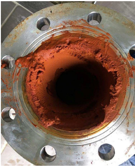
Fig. 5 Fe oxohydroxides precipitated inside a drop pipe section of a mineral water well
