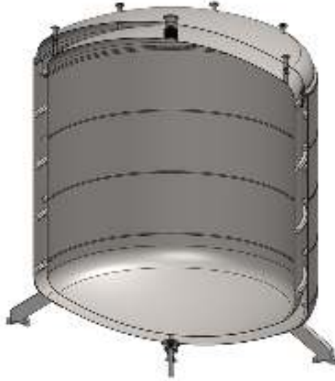
Fig. 11. 3D rendering of the DarkSide-20k cryostat.
