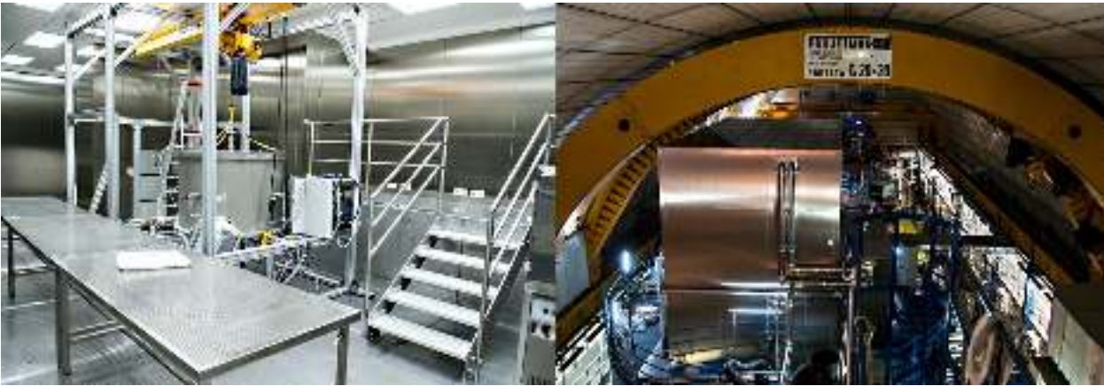
Fig. 96. The DarkSide-50 radon suppressed clean-rooms in Hall C . Left: The interior of the CR1 clean room, with the UHV evaporator for TPB coating of detectors' internals visible at left of center. Right: The exterior of the assembly clean room CRH on the top of the CTF water tank, housing DarkSide-50.
