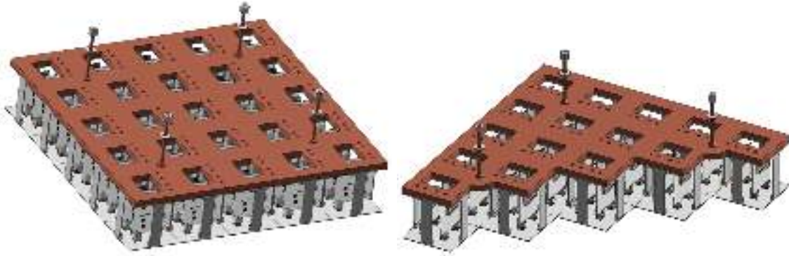
Fig. 50. Left: A single SQB (see text). Right: A single TRB (see text). SQBs and TRBs are assemblies of tiles serving as building blocks of the photon readout planes.
