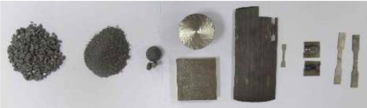
Fig. 12. Samples of ULR titanium at the different stages of production: 1. ULR titanium sponge; 2. magnetically separated crushed sponge; 3. isostatic compacted sponge; 4. vacuum arc-welded (cylinder) and electron-beam melted (rectangular block) ingots; and 5. samples for mechanical tests.
