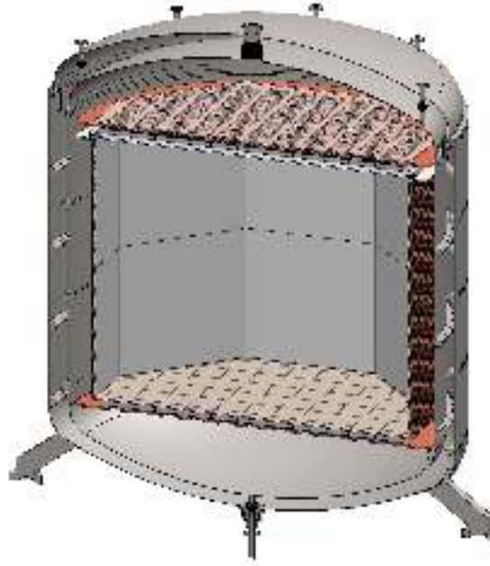
Fig. 44. 3D rendering of the DarkSide-20k LAr TPC and cryostat.
