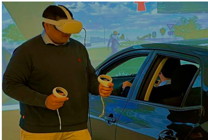
Fig. 7. Pedestrian and driver interaction in the multi-user simulator.
