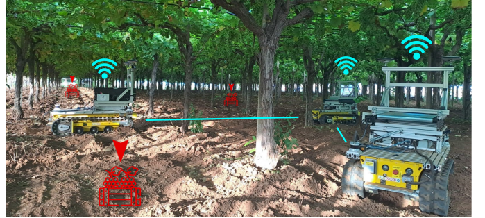
Fig. 1: Illustrative example of the operational scenario. Multiple robots communicate with each other and must perform services at scattered locations (red waypoints) across the field.
